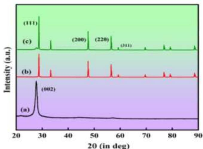
Figure 1: XRD pattern of (a) g-C<sub>3</sub>N<sub>4</sub>, (b) CeO<sub>2</sub>, and (c) g-C<sub>3</sub>N<sub>4</sub>/CeO<sub>2</sub> composite prepared via physical grinding
