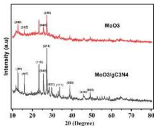
Fig. XRD patterns of MoO<sub>3</sub> and MoO<sub>3</sub>/gC<sub>3</sub>N<sub>4</sub>
