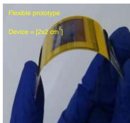
Fig.1: Electrodeposition of PEDOT film on flexible PET; Image- flexible electrochromic device
