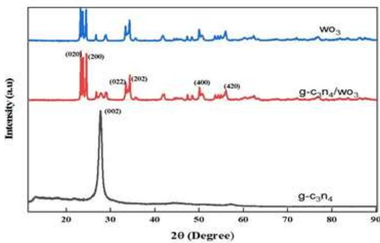
Figure 1: Comparison between the measured XRD pattern of g-C<sub>3</sub>N<sub>4</sub>, WO<sub>3</sub>, and g-C<sub>3</sub>N<sub>4</sub>/WO<sub>3</sub> composite synthesized via physical grinding for 2 h and heated at 500°C.
