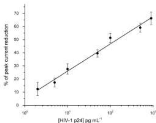
Fig.2 Calibration plot for the immunosensor
