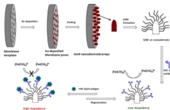
Fig.1 Schematic illustration of the different steps for the immunosensor construction
