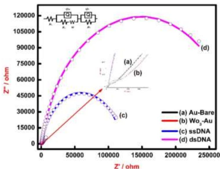
Figure 1- Electrochemical impedance behaviour of Modified gold electrode measured in PBS buffer (pH 7.4) in presence of 1mM K<sub>3</sub>/ K<sub>4</sub> Fe[(CN)<sub>6</sub>]<sup>3-/4-</sup> in the frequency range of 100KHz to 1KHz and applied potential 0.16v.
