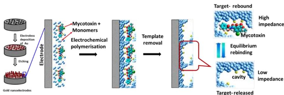
Scheme 1. Schematic representation of MIP sensor for Aflatoxin B1 fabrication and sensing mechanism.
