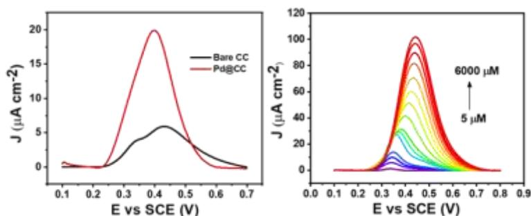
Figure: DPV response of bare CC and PdCC with the existence of 1 mM ACAP and (B) DPV concertation effect.
