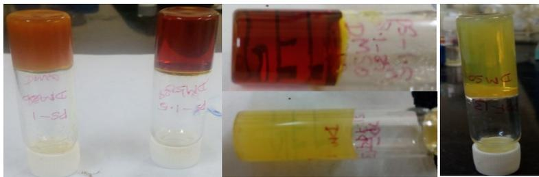
Figure. a) Inversion test of polymer gel derived from TAP and TPA in 1:1 and 1:1.5 molar ratio (from left to right) respectively; b) Transparency of PT- gel (upper) and PPF-gel (lower); c) inversion test of PPF-3-gel derived from TAP and Paraformaldehyde.
