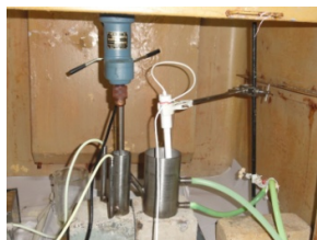
Figure. 1 Photograph of single stagemixersettler during uranus runs
